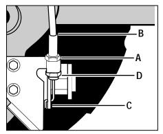
Figure 5-4: Wheel gear cable assembly.
